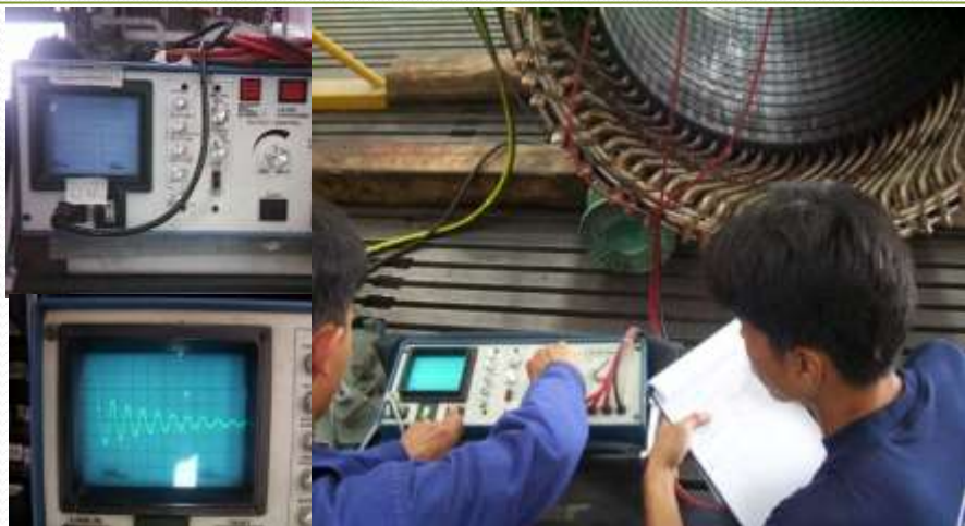
HV 12 KV SURGE COMPARISON TESTER& 12KVdc HIPOT
